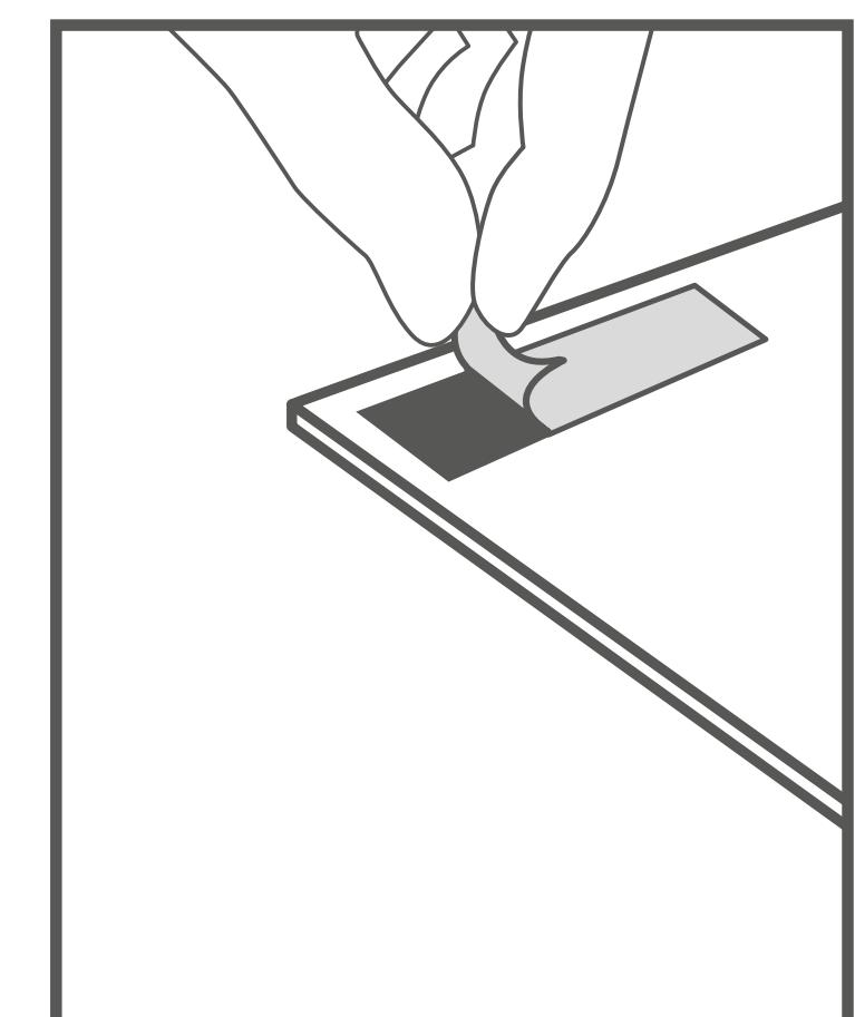
Unclip and place the back of the finishing trim against the wall. (Trim not included in the box)
